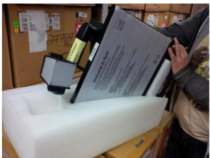
6. Remove remaining foam and film protecting monitor. Refer to the user manual for getting started with your new Smartview 360.
